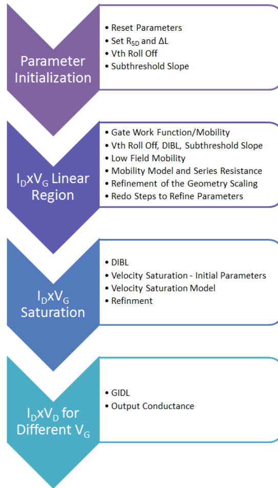
Figure 4.4: Simplified flow of the parameter extraction procedure for the BSIM-CMG model
