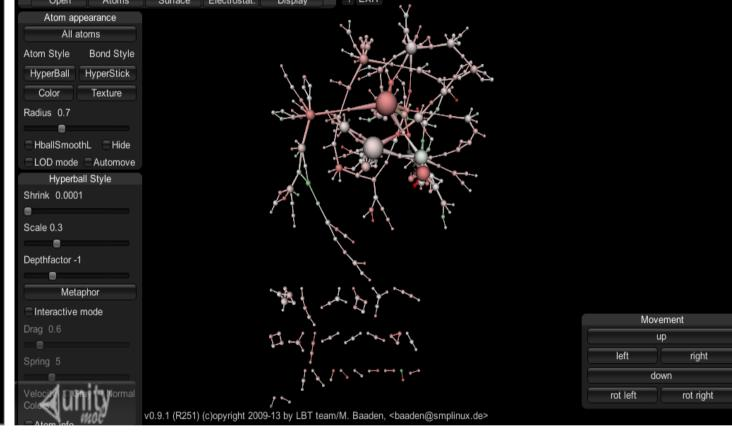
Spheres and cubes are used to render atoms (for molecular structures) or nodes (for networks); links between them are rendered using lines.
