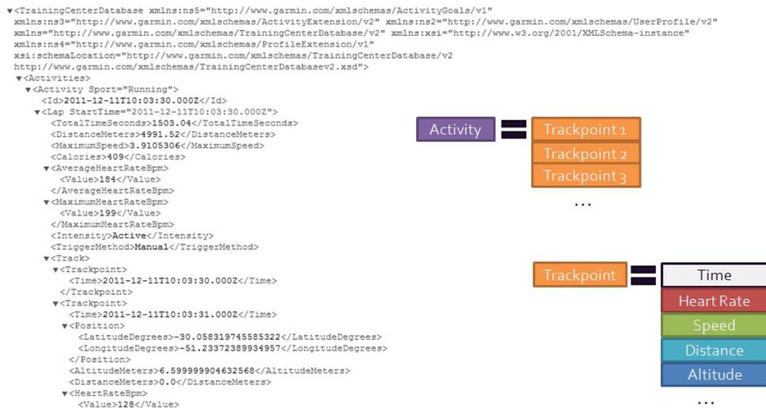
Figure 7.3: TCX file Structure of a TCX file. Each file represents an activity as a ordered set of trackpoints. Each trackpoint stores the value of a number of variables for a given unique timestamp.
