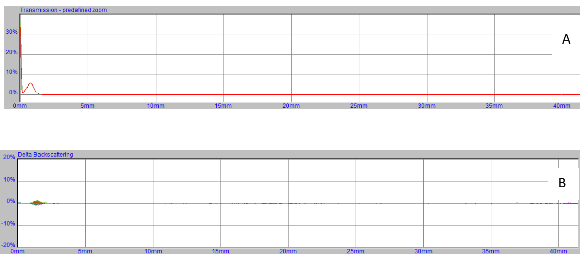
Figure 5. Analysis of transmission and of Delta Backscattering by Turbiscan LAb®. Intensity of transmitted light (A) and intensity of backscattered light (B) of Abisab/IndOH/IndOEt- NC formulation.
