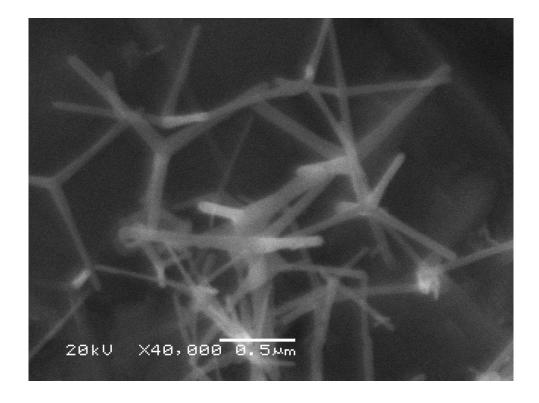
**Figure 1.** Scanning Electron Microscopy (SEM) of  $ZnO_{nano}$  showing the nanostructure after thermal evaporation process (40000x).
