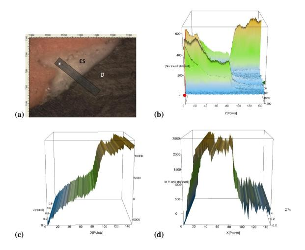
**Figure 3.** Interface analysis by micro-Raman. Representative Raman analysis of dentin-sealer interface. (a) Picture of the interface where ES is the experimental sealer, D is the dentine and the rectangle marked by \* is the representation of the analyzed line. (b) Overall interface analysis. (c) Graph representing the integration of the hydroxyapatite corresponding peak (910 cm<sup>-1</sup>). (d) Graph representing the integration of the corresponding zinc oxide peak (582 cm<sup>-1</sup>).
