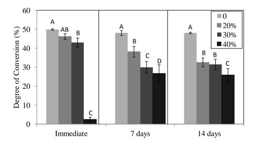
**Figure 2.** Degree of conversion of experimental sealers as a function of  $ZnO_{nano}$  concentration over time. Different letters indicate significant differences between different concentrations at the same time (p<0.05)
