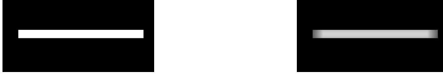
Figure 5.11: An ideal horizontal line (a) and its width estimates represented as intensities using K_u is shown in (b), where the wider the thickness measured, the higher the pixel intensity. Note in (b) the normalized width estimates decay at the extremities of the line.
