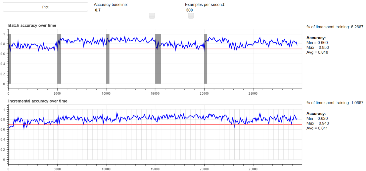
Figure 4.3 – A screen capture of the visualization developed to compare the behavior of batch and incremental algorithms. The shaded regions (which are very narrow and close to each other in the bottom half) correspond to time spent training a model. The overall proportion of time spent training is reported on the right side of the window.
