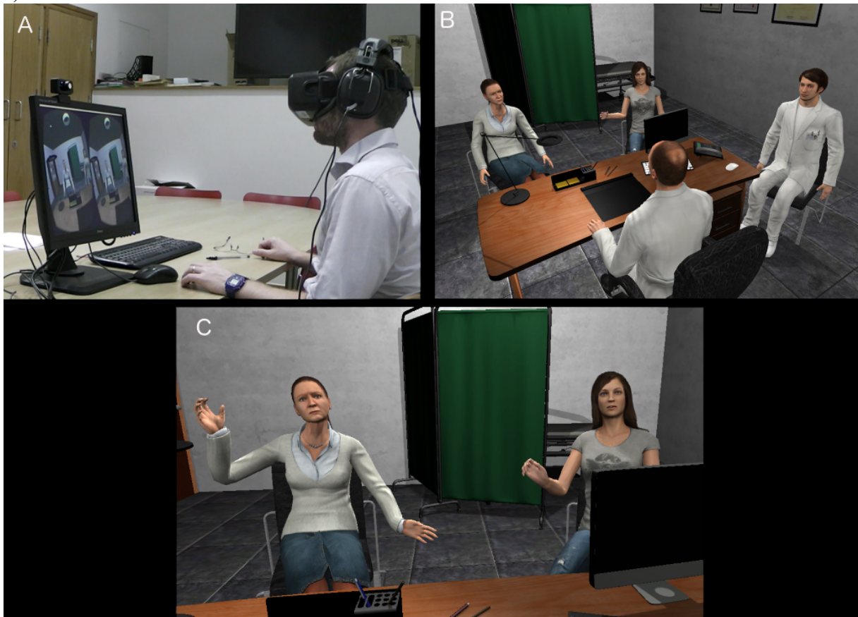
Figure 2.6 – Virtual reality set-up. a) the user wearing the HMD; b) an overview of the full VR scene; c) user's view in the VR world.
