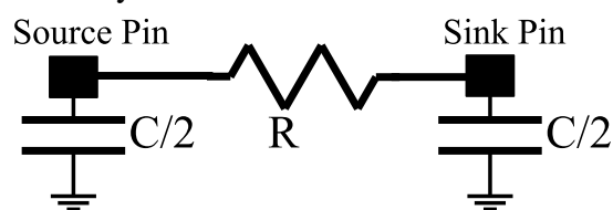
Figure 2.12: \pi wire model. Electric properties of wire segments are modeled with two capacitors that are connected by resistor
