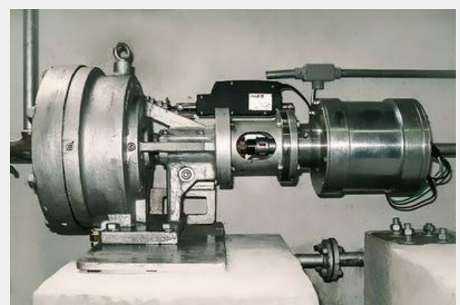
The Pressure Reducing Turbine (PRT) converts thermal energy that would be dissipated in pipe lines of huge electric power plants - Prosumir/Promotion
