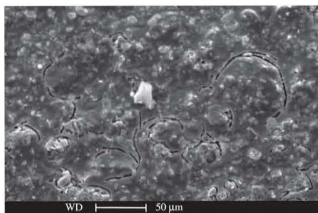
Figure 8. SEM photomicrograph of unpolished and non-etched glass porcelain surface, showing that crack bridging can occur due to the stresses released from large quartz particles.
