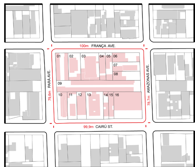
Figure 70. The floor plan for the sample block (in red in the middle) surrounded by nine facing blocks. Although the blocks have regular shapes, the building footprints show a random footprint.
