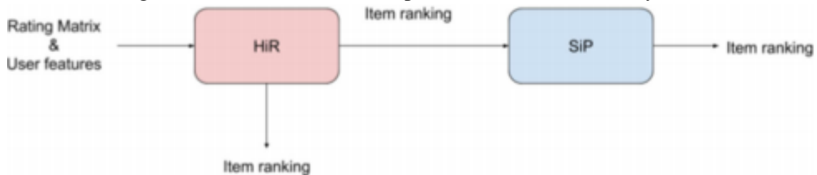
Figure 3.2: Architecture of the persuasive recommender system.
