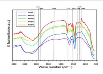
Figure 2: FTIR absorption spectra of the different produced MNPs, with stripes indicating important bands.
