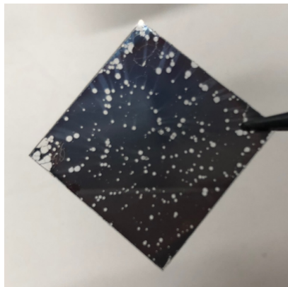
Figure 4.11: Typical perovskite layer deposited on a PTAA-covered ITO substrate, showing many holes caused by wettability problems.
