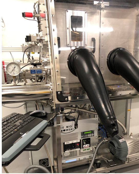
Figure 3.6: Picture of the evaporator (inside a glovebox) used to deposit LiF, C 60 and the Ag contact.
