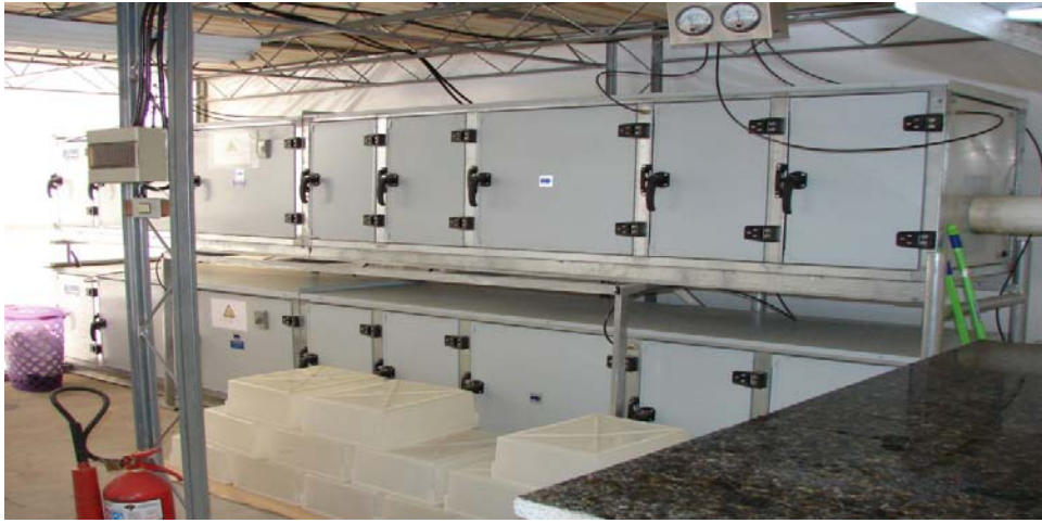
Figure 2. Internal view of the first floor of the exposition chamber with the air filter.
