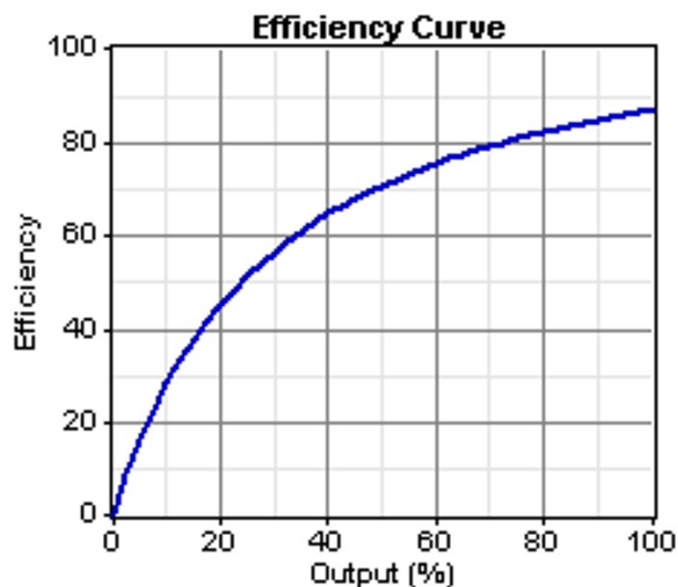
Figure 7.9: Efficiency as a function of the percentage of power supplied by the generator, simulating a compressed air turbine.
