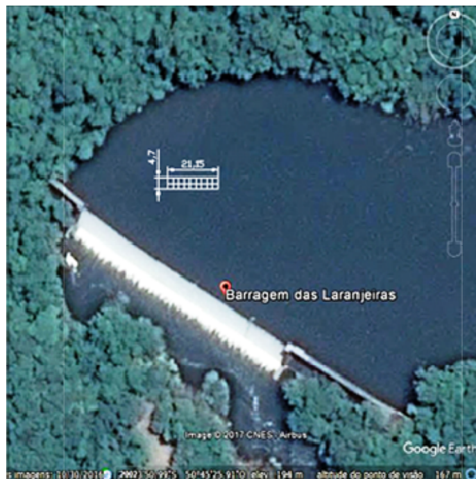
Figure 7.2: Image of the Laranjeiras Dam and comparison of the dimensions of the PV panels placed on floating structures with the region near the dam.
