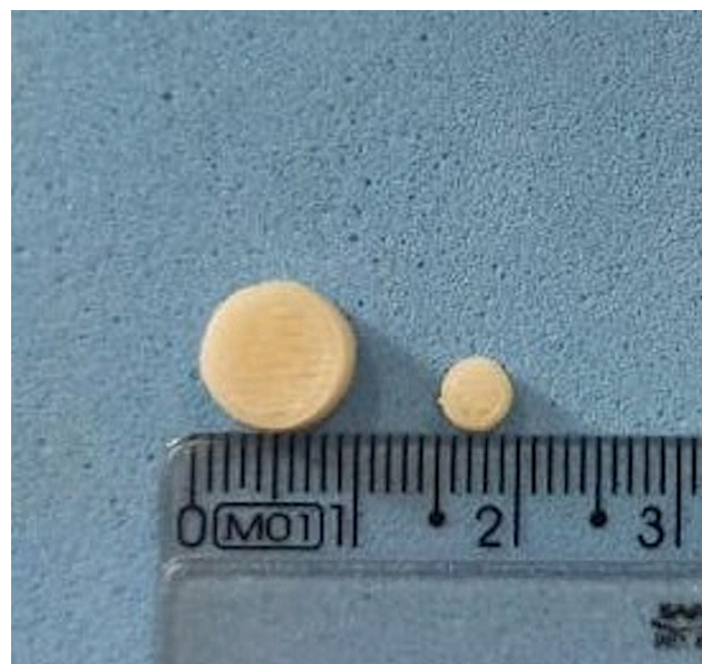
Fig. 2. 3D printed solid forms in two sizes: 10 × 3.6 mm – printlet (PRT); and 5 mm × 1.8 mm – mini-printlet (MPRT).
