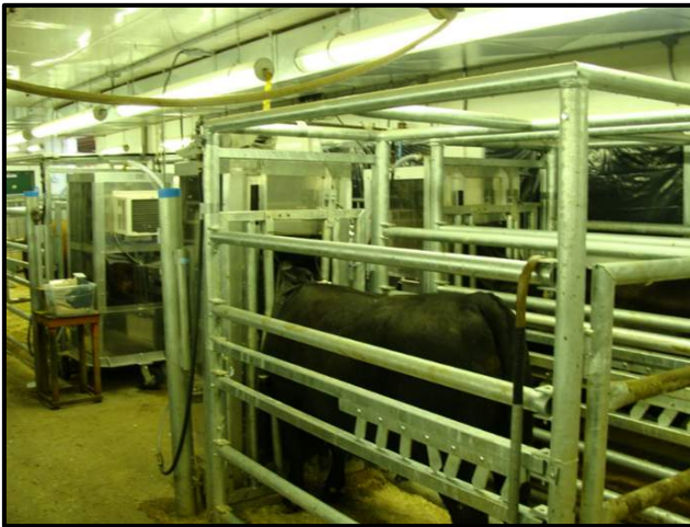
Figure 1. Indirect calorimeter system in operation. Note the neck sleeve fastened to minimize air leakage and allow cattle to stand or lay down. The head chambers were equipped with an air conditioner to condense water vapour from respiration and eructation. The system was also equipped with an 8,000 PPM carbon dioxide alarm to ensure animal welfare during the calorimetry assessment. Source: (Montanholi et al 2011).
