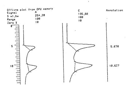
Figure 4.16 Digested Sludge Chromatogram – Capsule
