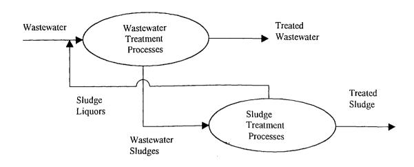
Figure 4.20 Wastewater and Sludge Treatment as a Feedback System
