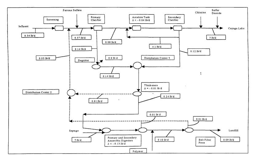
Figure 4.43 Mass Balance for Copper Associated with Solids-Bound Biopolymer at the Ithaca Wastewater and Sludge Treatment Plant – Average Values for June, July and August 1998.
