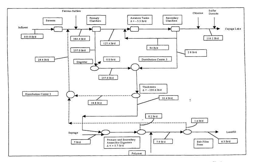
Figure 4.28 Mass Balance for Loosely-Bound Biopolymer Protein at the Ithaca Wastewater and Sludge Treatment Plant – Average Values for June, July and August 1998.
