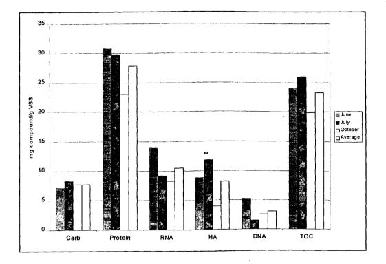
Figure 4.9 Weight Ratios of Capsular Biopolymers Constituents to Volatile Suspended Solids - Activated Sludge
