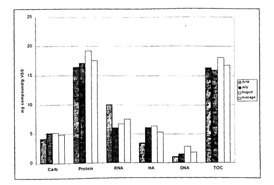
Figure 4.10 Weight Ratios of Capsular Biopolymers Constituents to Volatile Suspended Solids – Digested Sludge
