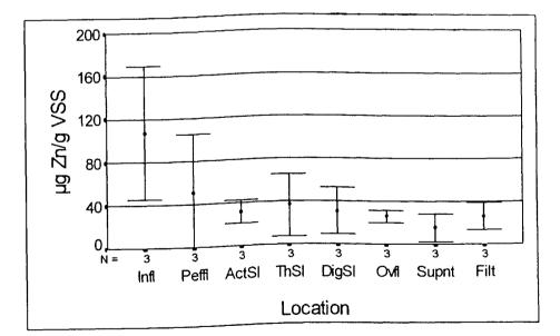
Figure 4.34 Ratio of Zinc in Solids-Bound Biopolymers to Volatile Suspended Solids
