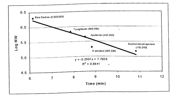
Figure 4.14 Molecular Weights Versus Elution Times for Standards
