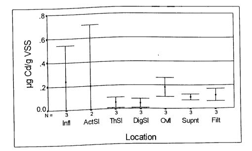
Figure 4.36 Ratio of Cadmium in Solids-Bound Biopolymers to Volatile Suspended Solids
