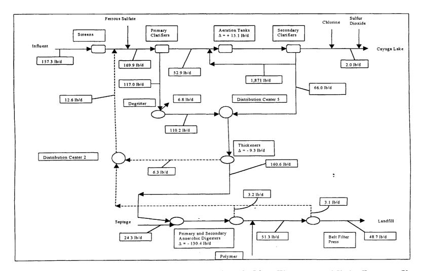
Figure 4.23 Mass Balance for Solids-Bound Biopolymer Protein at the Ithaca Wastewater and Sludge Treatment Plant Average - Values for June, July and August 1998.
