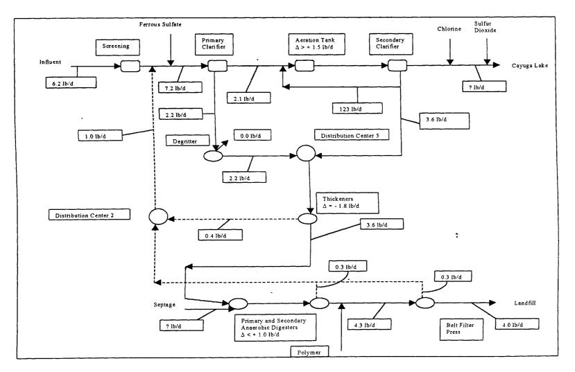
Figure 4.31 Mass Balance for Copper at the Ithaca Wastewater and Sludge Treatment Plant Average Values for June, July and August 1998.
