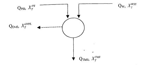
Figure F.9 Input to, and Output from, the Thickeners
