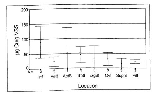
Figure 4.33 Ratio of Copper in Solids-Bound Biopolymers to Volatile Suspended Solids
