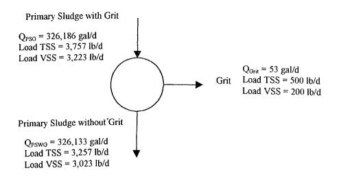
Figure F.3 Flowrates and Mass Balance for Suspended Solids on the Degritter
