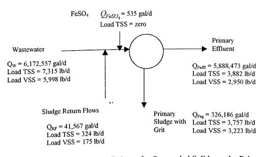
Figure F.2 Flowrates and Mass Balance for Suspended Solids on the Primary Sedimentation Tank
