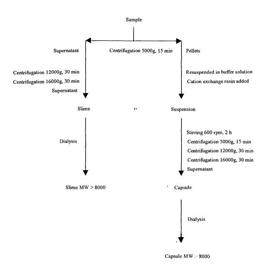
**Figure 3.2 Biopolymer Extraction Procedure**
