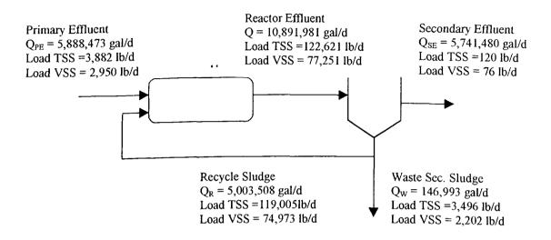
Figure F.8 Flowrates and Mass Balance for Suspended Solids on the Activated Sludge Process
