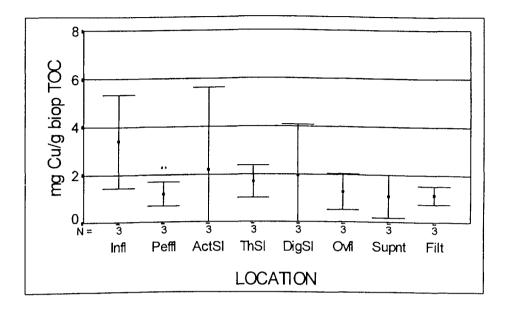
Figure 4.39 Ratio of Copper in Solids-Bound Biopolymers to Solids-Bound Biopolymers
