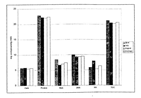
Figure 4.11 Average Weight Ratios of Capsular Biopolymers Constituents to Volatile Suspended Solids, in All Locations
