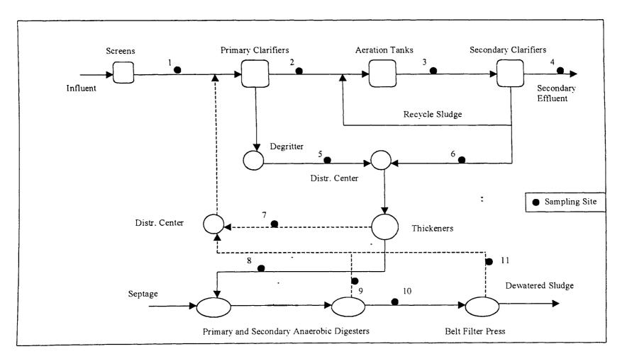
Figure 3.1 Sampling Sites at the Ithaca Wastewater and Sludge Treatment Plant
