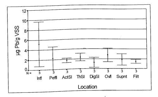
Figure 4.35 Ratio of Lead in Solids-Bound Biopolymers to Volatile Suspended Solids
