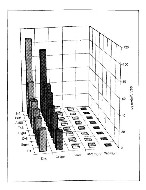
Figure 4.37 Weight Ratios of Trace Metals Bound to Capsular Biopolymer to Volatile Suspended Solids
