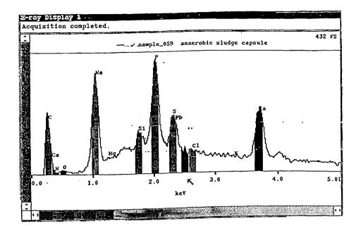
Figure 4.12 X-Ray Spectrum from Digested Sludge Capsular Biopolymer
