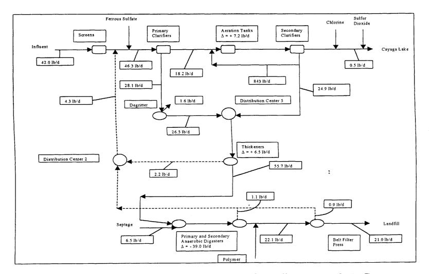
Figure 4.25 Mass Balance for Solids-Bound Biopolymer RNA at the Ithaca Wastewater and Sludge Treatment Plant - Average Values for June, July and August 1998.
