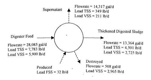
Figure F.11 Flowrates and Mass Balance for Suspended Solids on the Anaerobic Digesters
