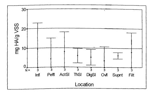
Figure 4.5 Humic Acids Content of Solids-Bound Biopolymers
