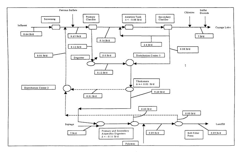
Figure 4.44 Mass Balance for Zinc Associated with Solids-Bound Biopolymer at the Ithaca Wastewater and Sludge Treatment Plant – Average Values for June, July and August 1998.
