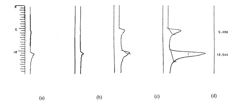
Figure 4.18 Slime Chromatograms – (a) Influent, (b) Activated Sludge, (c) Thickened Sludge, (d) Digested Sludge
