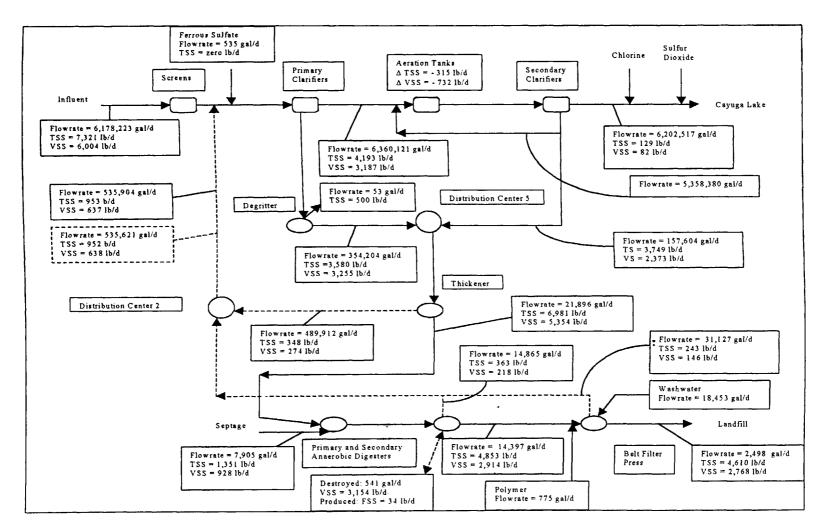
Figure 4.21 Flowrates, Total and Volatile Suspended Solids Mass Balance at the Ithaca Wastewater and Sludge Treatment Plant – Average Values for June, July and August 1998 (End of Fourth Iteration)
