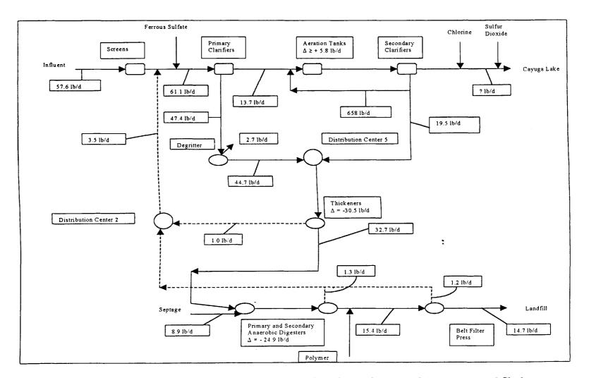
Figure 4.26 Mass Balance for Solids-Bound Biopolymer Humic Acids at the Ithaca Wastewater and Sludge Treatment Plant - Average Values for June, July and August 1998.
