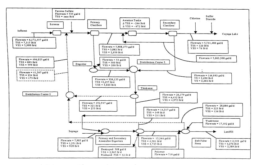
Figure F.13 Flowrates and Suspended Solids Loads in Wastewater and Sludge Treatment Processes at the Ithaca Wastewater and Sludge Treatment Plant (First Iteration)
