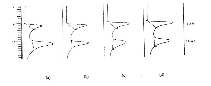
Figure 4.17 Capsule Chromatograms – (a) Influent, (b) Activated Sludge, (c) Thickened Sludge, (d) Digested Sludge
