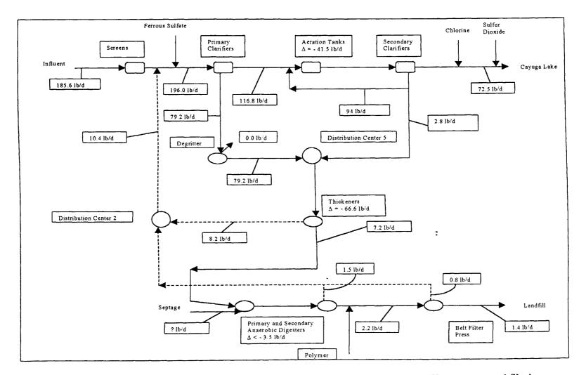
Figure 4.29 Mass Balance for Loosely-Bound Biopolymers Carbohydrate at the Ithaca Wastewater and Sludge Treatment Plant – Average Values for June, July and August 1998.
