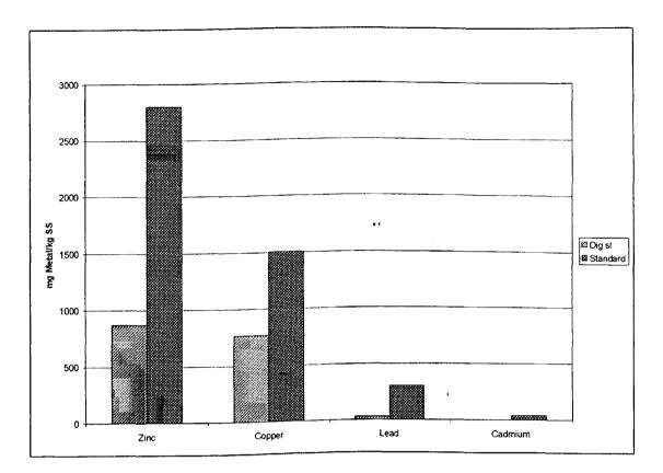
Figure 4.30 Trace Metals in Digested Sludge Solids and Standards for Exceptional Quality Sludges
