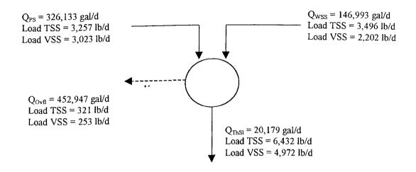
Figure F.10 Flowrates and Mass Balance for Suspended Solids on the Thickeners
