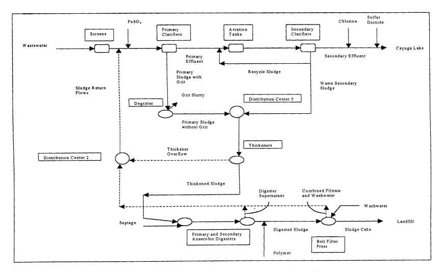
Figure 4.19 General Layout of the Ithaca Wastewater and Sludge Treatment
