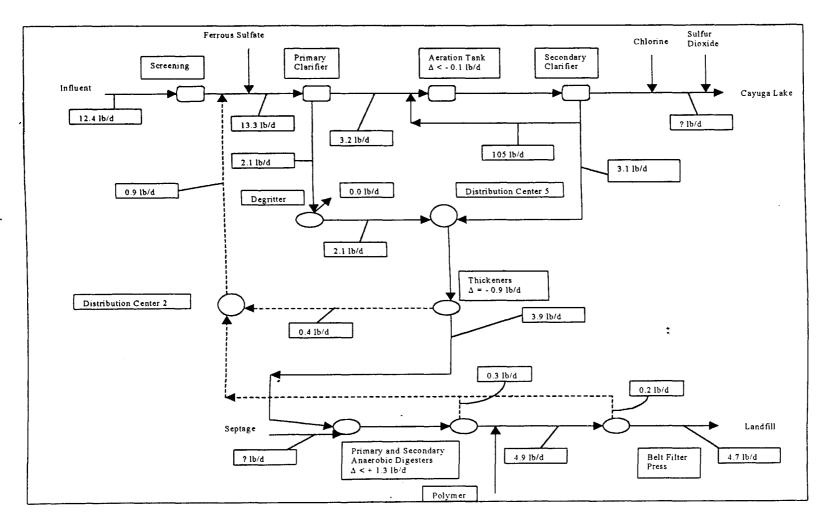
Figure 4.32 Mass Balance for Zinc at the Ithaca Wastewater and Sludge Treatment Plant Average Values for June, July and August 1998.
