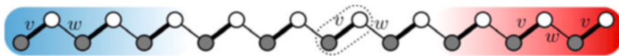
FIGURE 3.1. Schematic view of a Polyacetylene chain, taken from (1), with v/t = 1 + \delta the intra-cell hopping and w/t = 1 - \delta the inter-cell hopping amplitudes.
