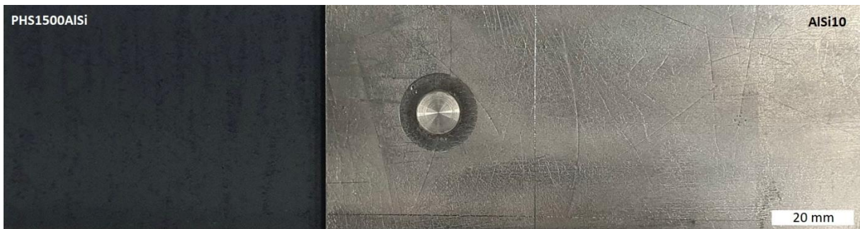
Figure 12 – A representative surface of overlapped AlSi10 welded to a PHS1500AlSi by RFSSW, highlighting the good surface finish. Source: the author.
