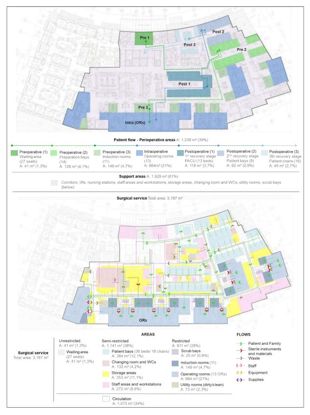
**Figure 1** – On the top: perioperative and support areas, the arrows representing patient flow. At the bottom: diagrams of areas, access restrictions, and flows.
