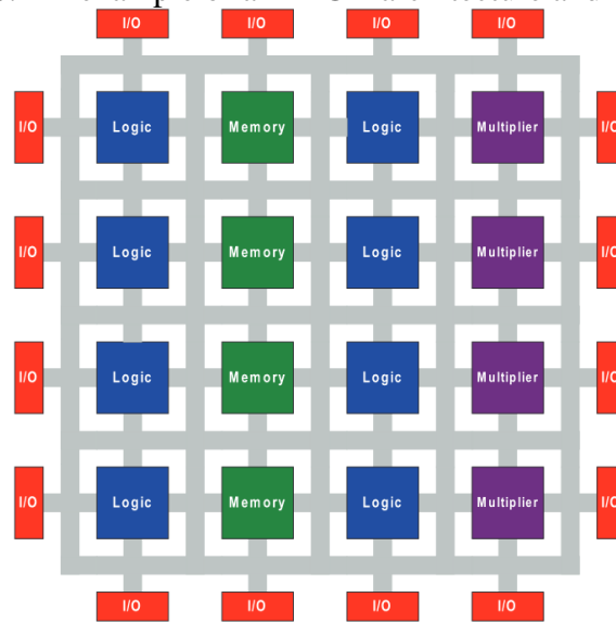
Figure 2.6: An example of an FPGA architecture and its resources.
