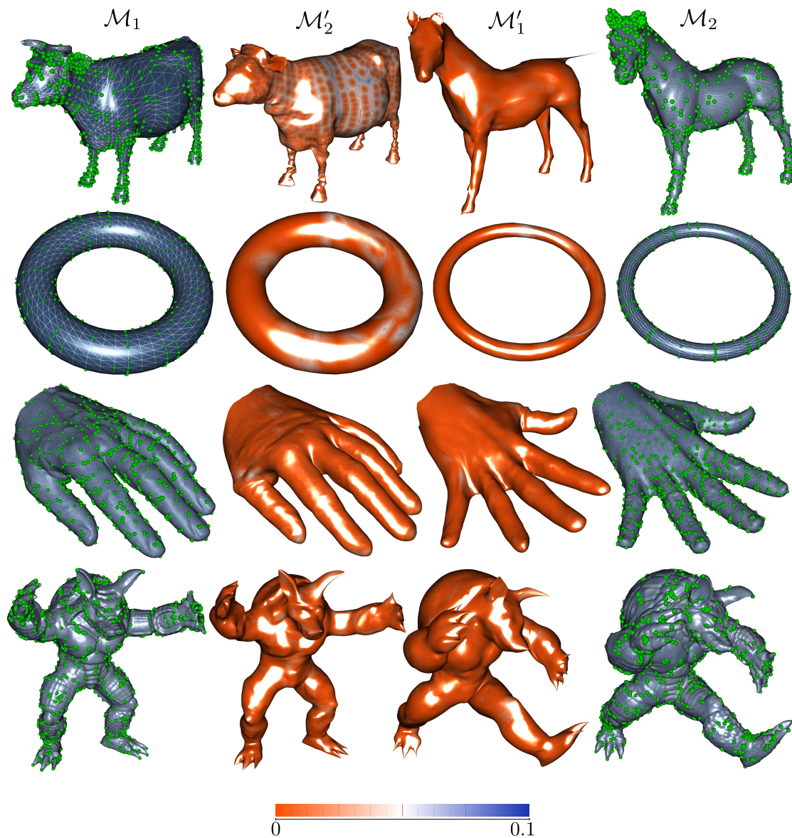
Figure 6.2: Surface Mapping Results. We have conducted four different mapping experiments, with varying models. The extreme left and extreme right columns illustrate the input meshes \mathcal{M}_1 and \mathcal{M}_2 , respectively. The center columns depict \mathcal{M}'_2 and \mathcal{M}'_1 , in this order. Observe how \mathcal{M}'_2 approximates the geometry of \mathcal{M}_1 and how \mathcal{M}'_1 resembles \mathcal{M}_2 . The colormap illustrates the geometric error of the approximations, normalized by the diagonal of each model's bounding box. Also, the final constraints are visible as green dots on \mathcal{M}_1 and \mathcal{M}_2 .
