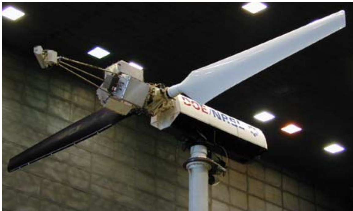
Figura 6.1 Turbina NREL Phase VI [Hand et al., 2001]
