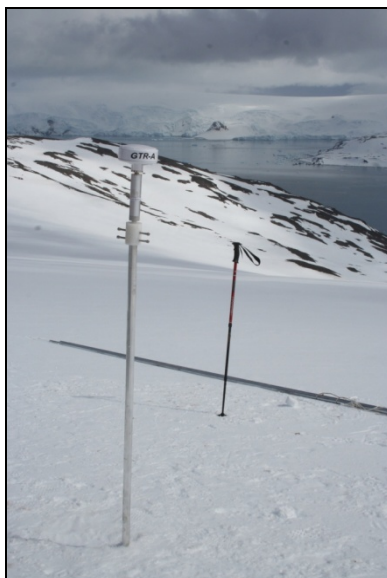
Figure 6 - Stakes along the Wanda Glacier central axis to determine surface ice velocity obtained in January, 2011 (Rosa et al, no prelo).
