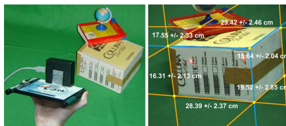
Figure 1. Scanner prototype: (left) Its operation. (right) Camera's view from another position showing the recovered dimensions and uncertainty computed in real time.
