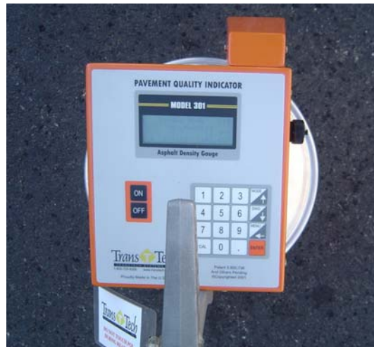
Figura 32: Equipamento Pavement Quality Indicator
