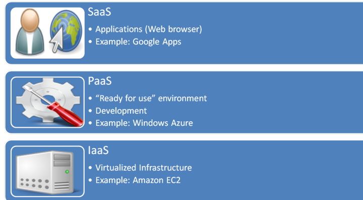
Figure 2.2: The cloud stack
