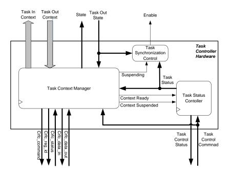
Figure C.1.: The controller template for a hardware task.
