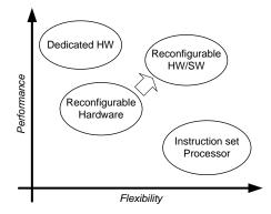
Figure 2.2.: Performance versus Flexibility tradeoff.
