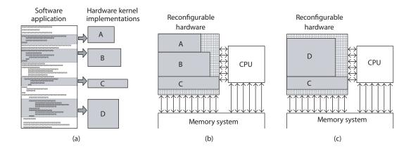
Figure 2.3.: Example of dynamic reconfiguration usage [33].
