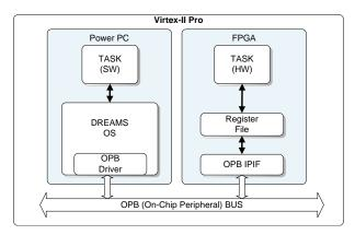
Figure 8.1.: Virtex-II Pro hardware/software interface.
