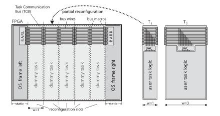
Figure 3.6.: OS frame and task communication block [114].
