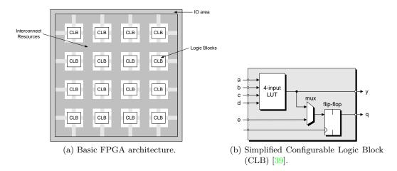
Figure 2.6.: FPGA comprises a set of CLBs.
