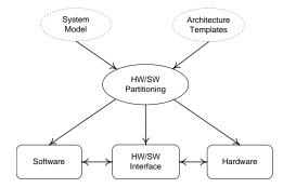
Figure 2.1.: HW/SW partitioning scheme.
