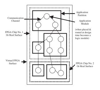
Figure 3.5.: A task graph on FPGA [98].
