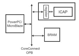
Figure 3.2.: Self-programming hardware architecture [87].
