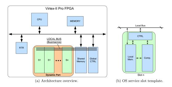
Figure 4.4.: System architecture.
