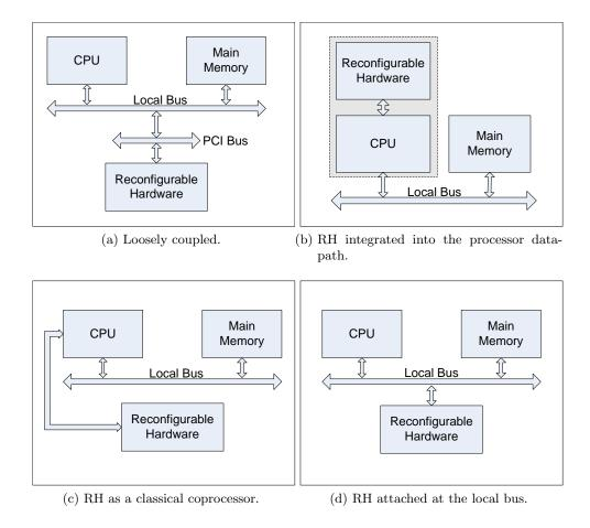
Figure 2.4.: CPU and RH: Coupling types.
