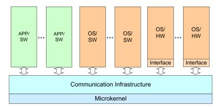
Figure 4.2.: Proposed microkernel based architecture.
