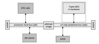
Figure 9.4.: Basic hardware platform.
