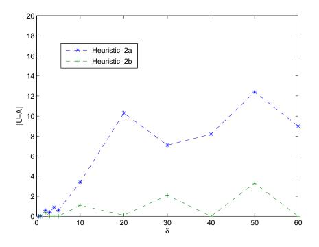
Figure 7.4.: Unbalance average for different  $\delta$  constraints.
