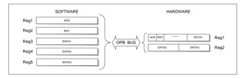
Figure 8.2.: Mapping between physical and virtual registers.
