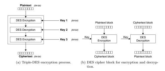
Figure 9.1.: Triple-DES and its basic DES cipher block.
