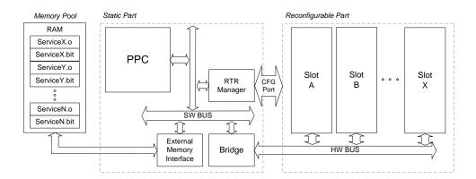
Figure 5.1.: System architecture highlighting the communication channels.
