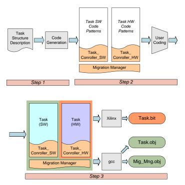
Figure 8.5.: Design flow supported by the framework.
