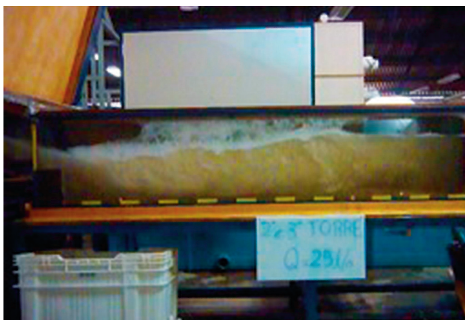
Figure 8 Passage of ten thousand-year floodwater (flow rate of 25 l/s, corresponding to the model value), simultaneously through the sill of tower 02 and side of tower 03- view from the transition box.
