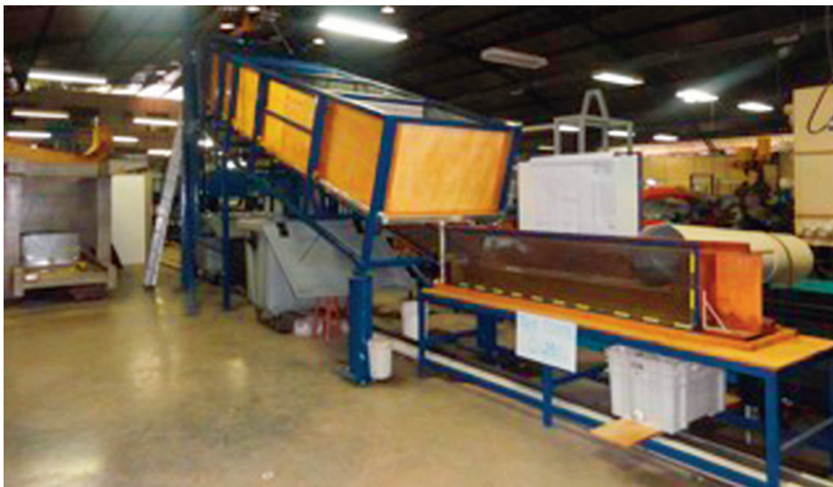
Figure 6 Hillside culvert connected to the outlet pipe
