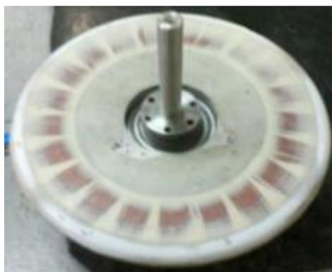
Figura 28 - Estator Enersud
