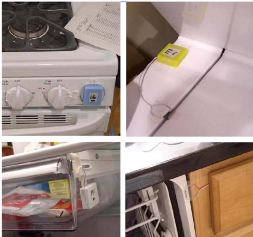
Figure 1.1: Example of binary sensors deployed in smart homes. MIT House_n Consortium
