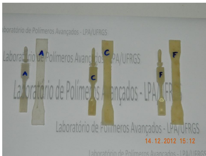
Figura 14 - CP's de PP (A) e Nanocompósitos de PP com NT's, (C) 2% cF, (F) 5% cF.
