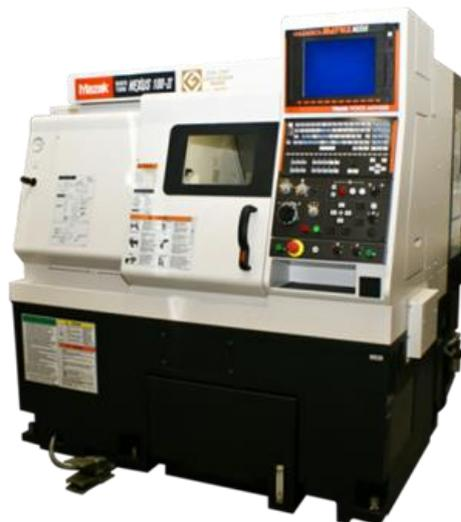
Figura 3.4 – Torno CNC Mazak QTN 100-II.
