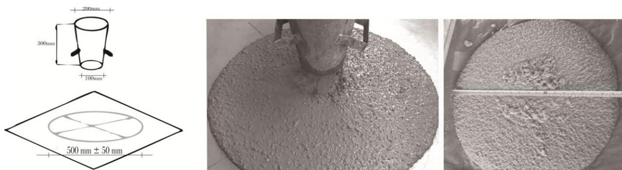
Figura 14. Slump Flow.
