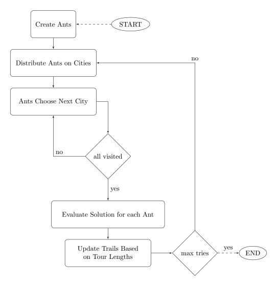
Figure 5: ACO for TSP Fluxogram
