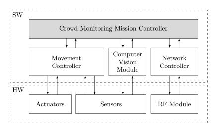
Figure 6: Solution Context and its Interface with Other Modules
