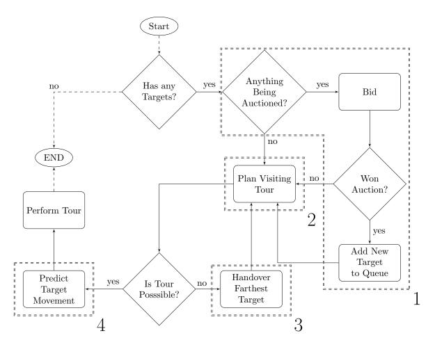
Figure 8: Detailed Flowchart of the Proposed Solution
