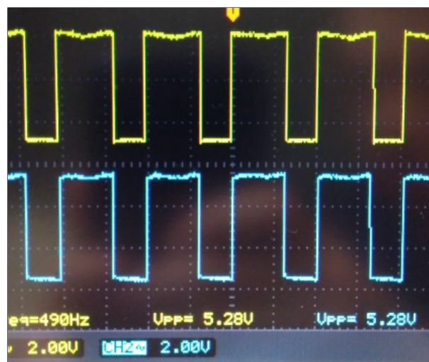
Figure 48. Left and right PWM: +2° steering wheel angle
