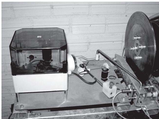
Figure 1. Braking system of Wind Energy Converter (WEC).
