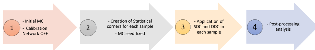
Figure 6. High-level simulation flow adopted in the assessment of SDC and DDC techniques.
