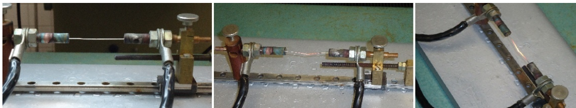
Figure 3.8 Thermocouple welding device. The images sequence: thermocouple wires alignment; star of welding process and; end of welding process.
