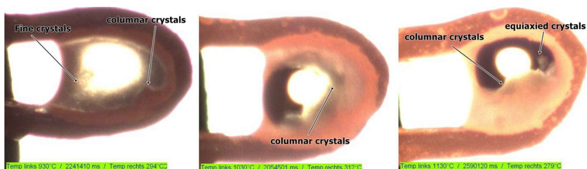
Figure 4.1.22 Crystal morphology of the CSA_M samples at 930°C, 1030°C and 1130°C, respectively.
