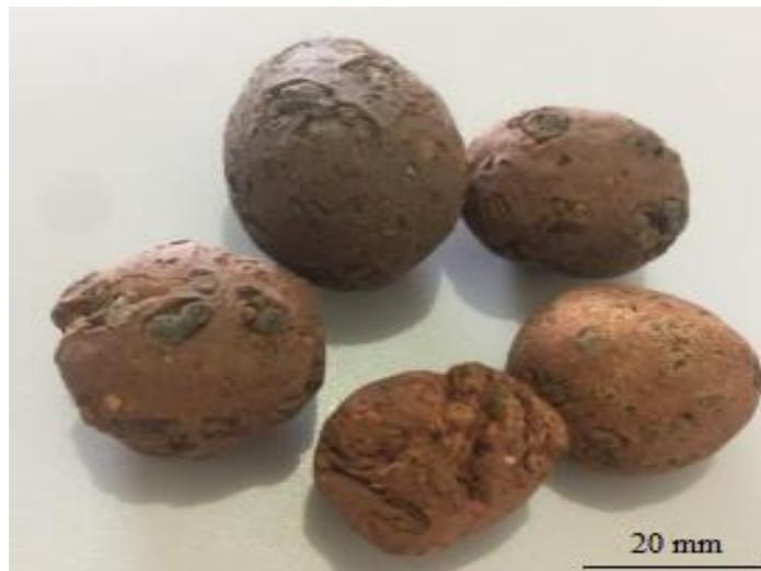
**Figure 1: Commercial light expanded clay aggregate.**
