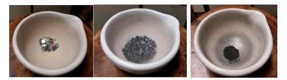
Figure 1. Grinding of NdFeB magnets from mobile phone devices with a mortar.
