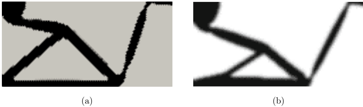
Figure 5.2 – (a) Final result of topology optimization and (b) an inverter obtained by Wang et al. [2017]
