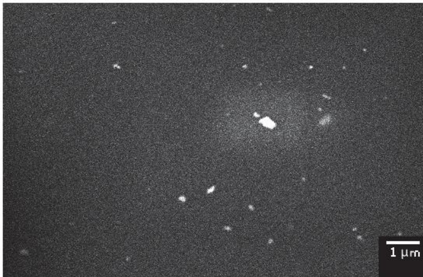
Figure 4.38: ZnO agglomerated nanoparticles on a PVP layer (in detail).
