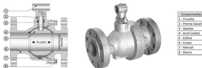
Figura A.2 - Válvula Esfera de construção *trunnion*
