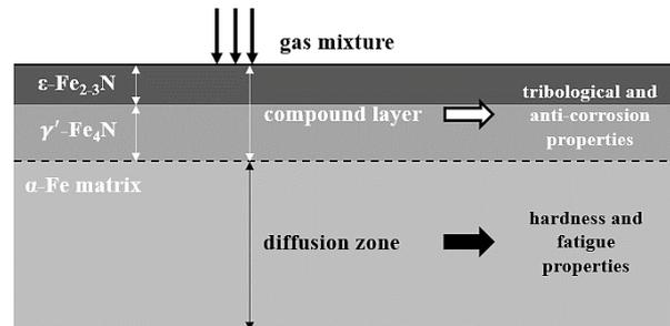
**Fig. 6:** Schematic Illustration of the Nitrided Zone of an Iron-Based Workpiece. The Nitrided Zone Can Be Subdivided Into the Compound Layer and Diffusion Zone. Reproduced from [101].
