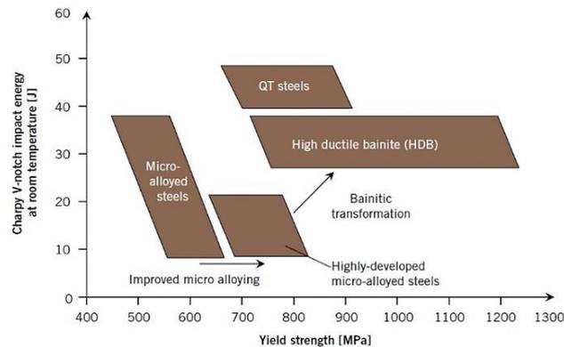
**Fig. 1:** Main Steel Types Used in the Manufacturing of Parts for the Automotive Industry. Reproduced from [4], [13].
