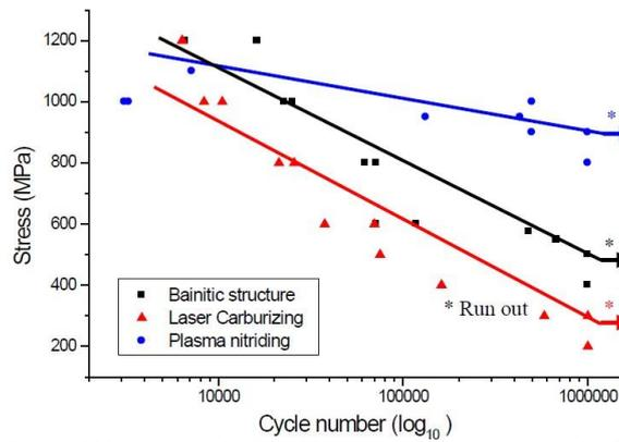
**Fig. 7:** Fatigue Curves (S-N) for the Conditions: 300 M Steel with Bainitic Structure and Steel with Surface Treatment of Plasma Nitriding and Laser Carburizing. Reproduced from [20].
