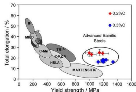
Fig. 3: Yield Strength and Total Elongation of Advanced Bainitic Steels In Comparison with Other Commercial Steel Grades. Reproduced from [57].
