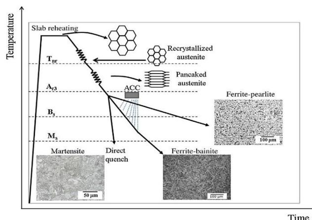
**Fig. 2:** Schematic of Microstructure Evolution in TMP Steels ( $T_{nr}$ : Nonrecrystallization Temperature;  $A_{r3}$ : Transformation Start Temperature;  $B_s$ : Bainite Start Temperature;  $M_s$ : Martensite Start Temperature. Reproduced From [52].
