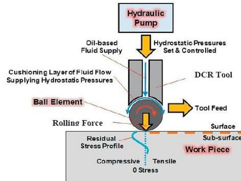
Fig. 4: Working Principles of Deep Rolling Process. Reproduced from [89].
