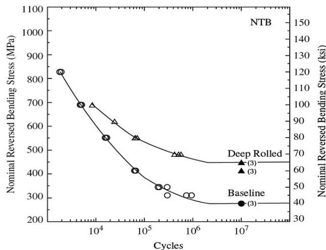
Fig. 5: A Comparison of Deep Rolling and Baseline Bending Fatigue Behavior for the Bainitic Direct-Cooled NTB. Reproduced from [39], [40].
